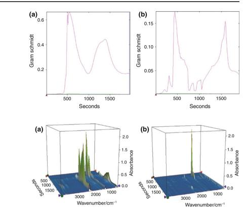
Fig. 4 3D FTIR plot during thermal degradation(a) combustion (b) pyrolysis
