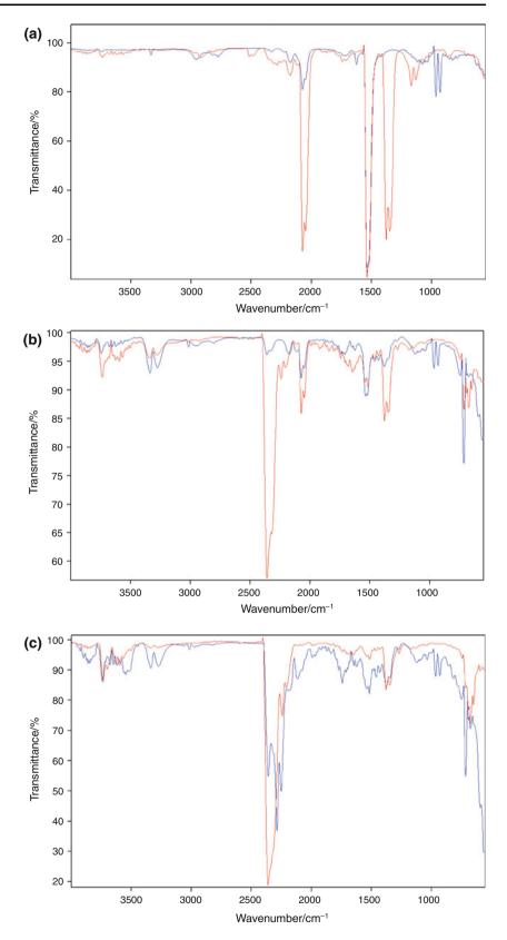
**Fig. 6** *Bar Graph* of the fragments originating in the thermal degradation at 500 °C (**a**) combustion (**b**) pyrolysis
