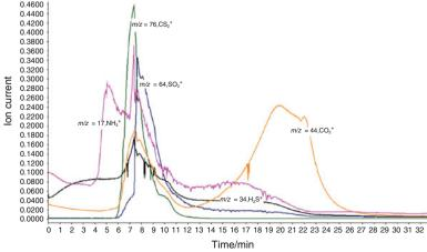
degradation is supported by the fragments at m/z 34, 32, and 33 [20]. The releasing of water begins at 80 °C and show fragments at m/z 18 in the first and second degradation stage during pyrolysis and combustion of TFR.
